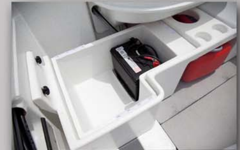
Stern bench seat. Incorporating battery locker, fuel storage, and dry storage or live bait well.
