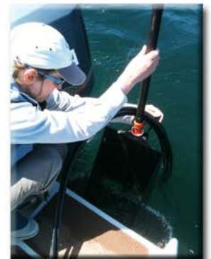
4 element HF hydrophone deployment on custom made mounting bracket. Denmark
