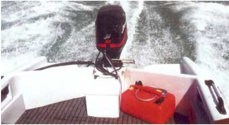
Note: Aluminium powder coated battery box, handrails, 'Autex' marine carpet. The 25-litre tote tank can be installed under the seating if preferred.
