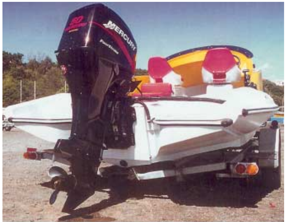
Note: How the pontoon hull extends out from the conventional hull shape providing substantial buoyancy and stability, also note how the portofino extension angles up and away from where it meets the main hull. This greatly assists with getting up on the plane with a heavy load on board.
